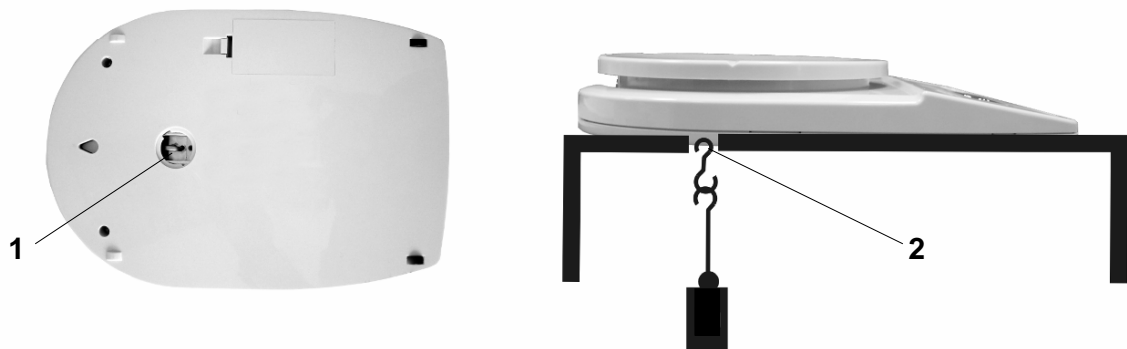
Fig. 1: Setting up the balance for underfloor weighings
